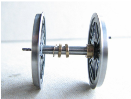
Assembled wheels for front or centre. Note from left to right on the axle; 1x0.25mm spacer plus 2x1mm spacers. And the same on the other side of the axle.
