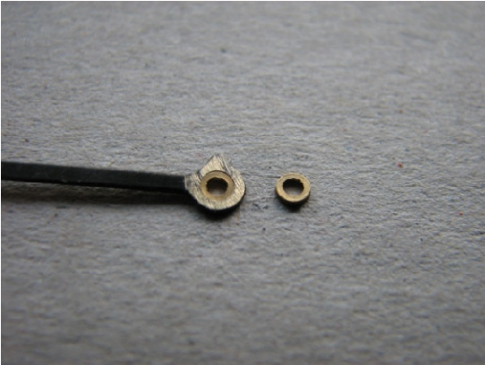
Bush in rod ready for soldering.
