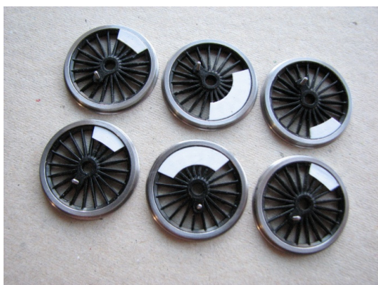
Wheels complete with weights and crankpins.
