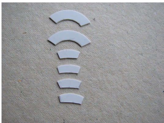
Balance weights cut from plasticard.
