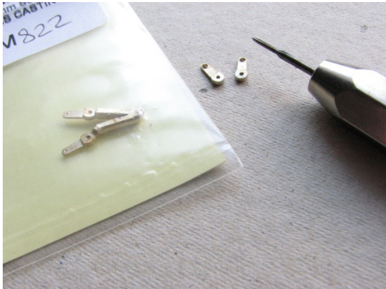
Return cranks as supplied with a prepared pair and tap alongside.
